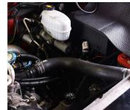
Remove the four bolts securing the bracket for the air box tray and degas bottle from front core support using a 13mm socket/wrench. (Two are located on the bottom of the bracket, two are up top). (Figure 7)
